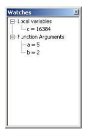
The arguments a and b are shown in the Watches window. Notice that the local variable c, which has not been set yet, has a random value.
