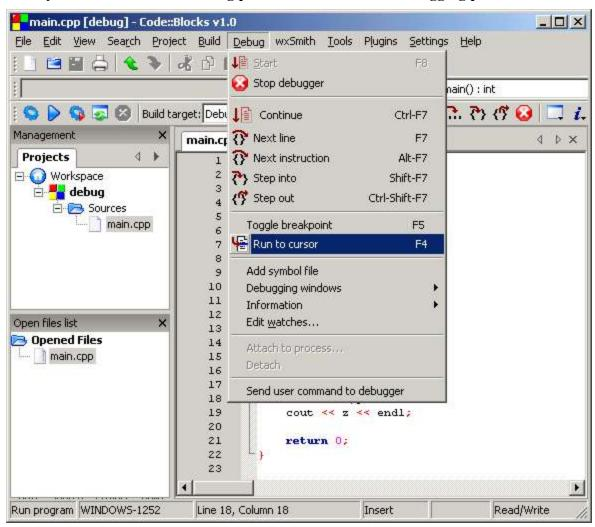
The next step in debugging a program is to tell the program when to stop running so you can inspect the results. To do this, place the cursor over the line where you want your program to stop. For example, the cursor was placed at line 18 (which is hidden behind the menu). This is called a **Breakpoint**. Now you can instruct the debugger to run the program up to the cursor's position (line number).
