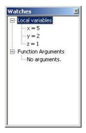
These are the watches that the debugger is displaying. Notice that  $\times \& y$  have the correct values. Variable z has not been assigned it's value on line 18 yet. The current value is a random value.
