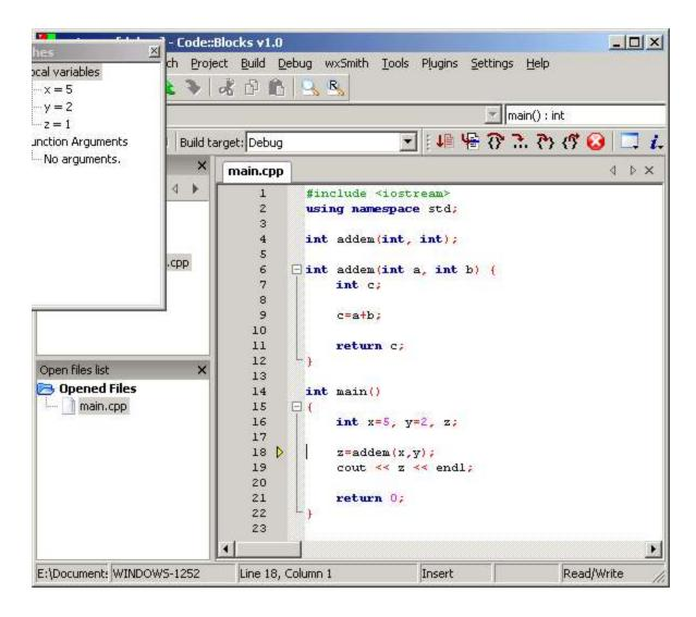
Line 18 has a yellow marker on the left side. This indicates that the program has paused on that line, which is the breakpoint.
