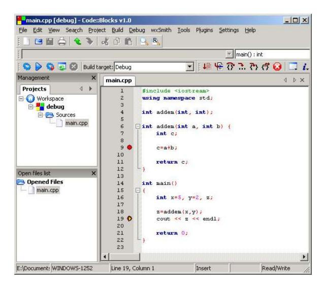
Now the program stops at line 19, because the program reached the second breakpoint. Press Ctrl-F7 to continue. Now the program runs till the end of the program, because there are no further breakpoints to encounter.
