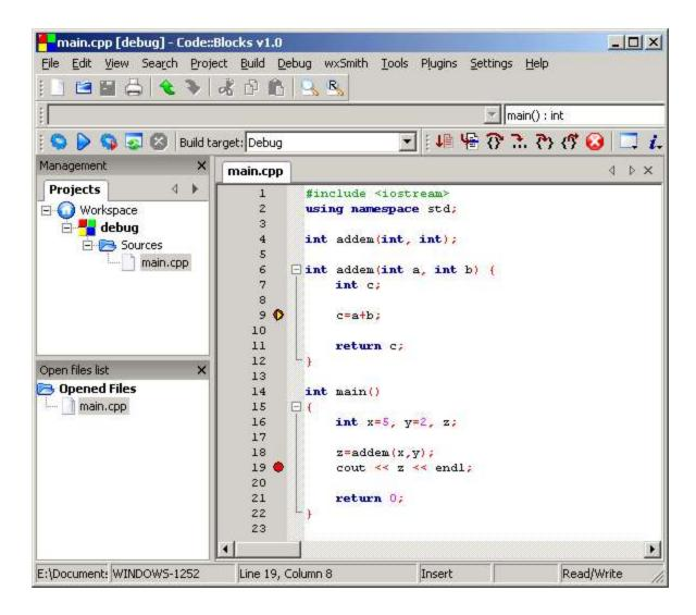
This screen shows breakpoints on lines 9 and 19, but line 9 indicates that the code has executed to that point.
