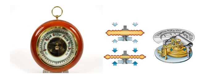
This is an instrument for measuring pressure without involving any liquid, invented in France by Lucien Vidi in 1844.
