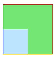
here the yellow line correspond to an artificially created boundary,  $\Gamma_3$ , where we assume homogeneous Neumann condition in order to ensure thermal insulation (i.e. no heat flux). The problem reads now
