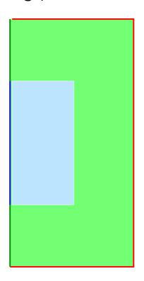
The light blue region,  $\Omega_0$ , is the interior of the refrigerator. The green one,  $\Omega_1$ , corresponds to the sides and the door of the fridge.  $\Gamma_0$ , in blue, is the refrigerated wall,  $\Gamma_1$ , in red, is the boundary at room temperature and  $\Gamma_2$ , in green, is part of the boundary where we suppose the temperature varies linearly.
